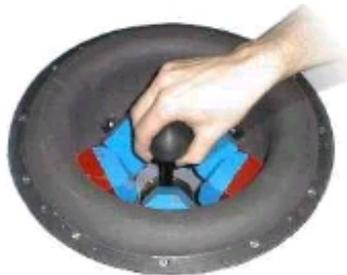
Abb. 16: Magnetic Levitation Haptic Device
